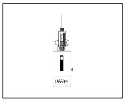
6) Regulate the dose using the dose regulator. To do so, screw or unscrew the dose regulator until it reaches the desired point on the dose scale. If, for example, you want to regulate the dose to 1.2 ml, you must bring the upper side of the dose regulator exactly to the 1.2 ml mark of the dose scale.
