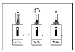
3) Again using the needle connector handler, screw the needle connector to it's original place.
