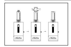
1) Using the needle connector handler, unscrew the needle connector.
