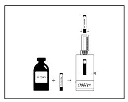
2) Wipe the cap of the PRL cartridge with alcohol and insert it into the cartridge compartment.
